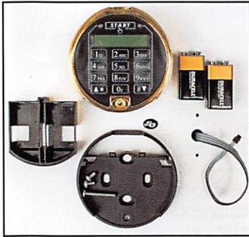
Here are the components of a Biometric Keypad kit. Note that it comes complete with batteries. The cable for an existing lock is shown coming through the spindle hole of a safe door.
