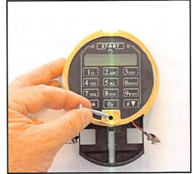
With the keypad mounted on the base, loosely install the long screw as shown. Do not tighten it until you have attached the batteries to the connectors and pushed the battery box into the keypad. After the screw is tightened, the self-stick S&G logo can be installed over the screw head.
