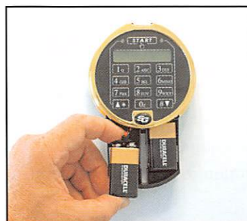
Battery replacement is simple. Just pull down on the battery box, remove the old batteries from the connectors, clip on new batteries, then push the box back up into the keypad housing.
